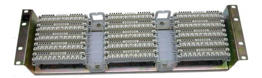
Recessed Subrack fitted with upto 3 nos of 5 way Back Mount Frame (BMF). This can be mounted on a 19" rack. A maximum of 15 Nos of 2/10 LSA-PLUS® Disconnection modules can be mounted on this to offer upto 75E1 terminations.
