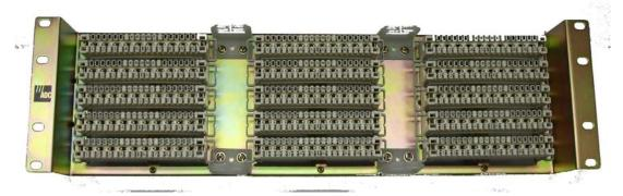
Recessed Subrack with inbuilt Back Mount Frame (BMF) can be mounted on a 19" rack. A maximum of 15 Nos of 2/10 LSA-PLUS® Disconnection modules can be mounted on this to offer upto 75E1 terminations.
