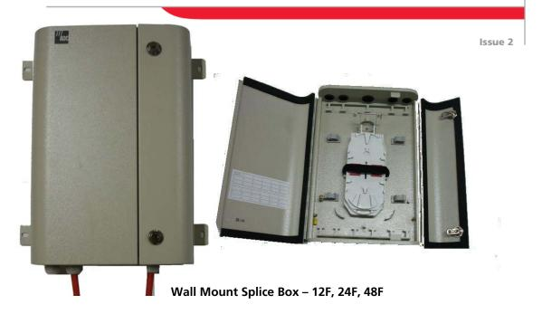
ADC's Wall Mount Fibre box provide fibre splicing capability interfacility. Fibre cable & fibre optical terminal patchcords in small & medium sized fibre network & customer premise application. Radius limiters used to maintain a protective minimum bend radius for patch cords bundles wound around in the storage spool.
