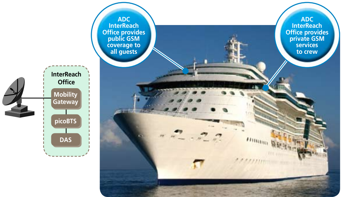
Ship network Scenario 1: large ships with local switching
