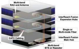
With a minimum of components and use of industry-standard 75 ohm CATV cabling, InterReach Fusion is simple and inexpensive to install, especially compared to heavy, inflexible, and invasive coaxial cabling. In addition, because power for the Remote Access Units is provided over the CATV cabling, no local power is required, further simplifying installations.
