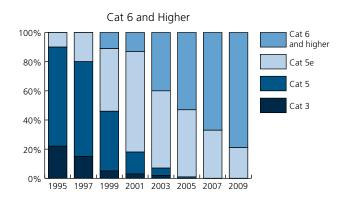
The second chart above shows how historically the cabling Category installed has always led well before the speed of the protocol supported is used. For example, in 1995 the primary UTP cabling being installed was Cat 5, which could support 100Mbps, but the switch ports sold that same year were primarily 10Mbps. In 1999 the primary switch port speed sold was 100Mbps, but the primary cabling solutions, Cat 5e and Cat 6, supported 1000Mbps.
