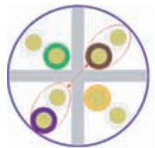
The star filler used within several Category 6 cable designs increases and controls the distance between pairs.
