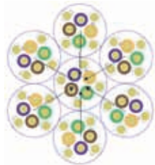
Example of a centre cable being impacted by the adjacent 6 cables in the bundle.
