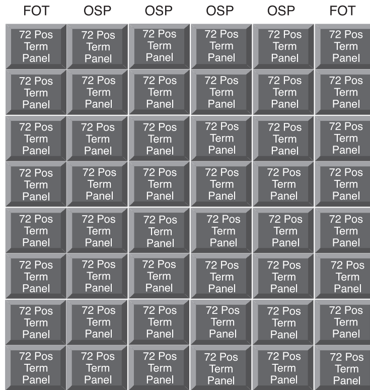
Figure 16. ODF cross-connect configuration with 2:1 OSP:FOT ratio
