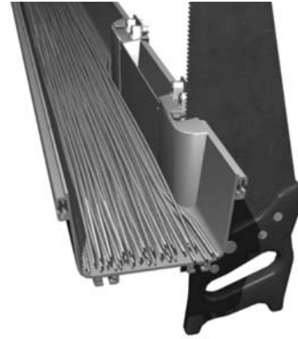
Fixture protects cables during cutting of sidewall
